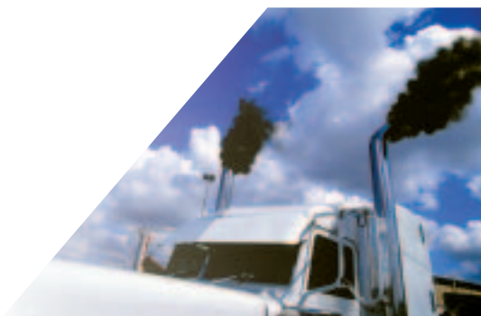
Particulate matter consists of soot or unused fuel found in exhaust. This type of pollution gives dirty engine exhaust its black color.
